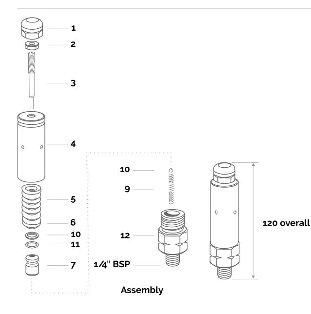
PED requirement: The valve body to be pressure tested to 1.5 maximum WP before assembly.
